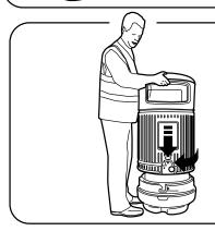
Lift body over liner and lower to rest on plinth, turn body clockwise to lock.
