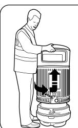
With the key still in position, turn body counter-clockwise, and lift body over liner. (See note A)
